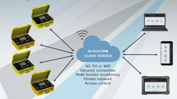
The AERO CLOUD BONDING app gives you the possibility to supervise several hot bonders at once remotely on different devices, via a private and secure cloud server.
